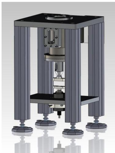
Multifrequency cavitation device
